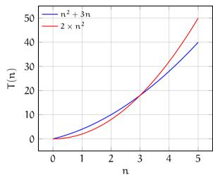
$$T(n) < 2 \times n^2 \text{ for } n \geqslant 4$$
